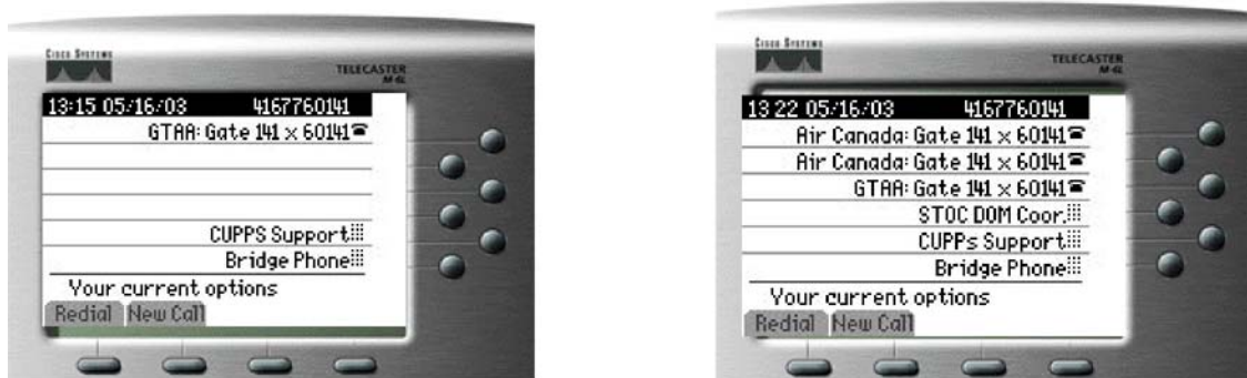
Figure 1. Gate Agents Can Log into any Cisco IP Phone to Personalize It with Their Airline's Phone Number, Directory, and Other Options
