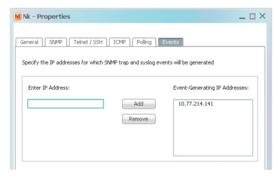
Logging should be enabled on Nexus 7000 (default vdc as well as non-default vdc's) and add the IP address of Cisco Prime Network Server as logging server host.
