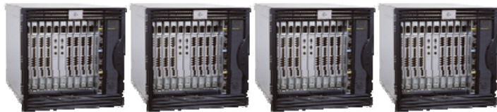
4x Brocade 24K with 16-Port 2G Modules
