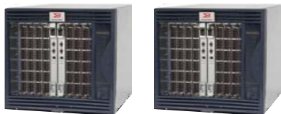
2x Brocade 48K with 16-Port 4G Modules
