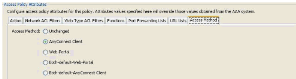
Figure 36. Access Method Tab—This configuration is necessary for defining the SSL VPN client connection types.
