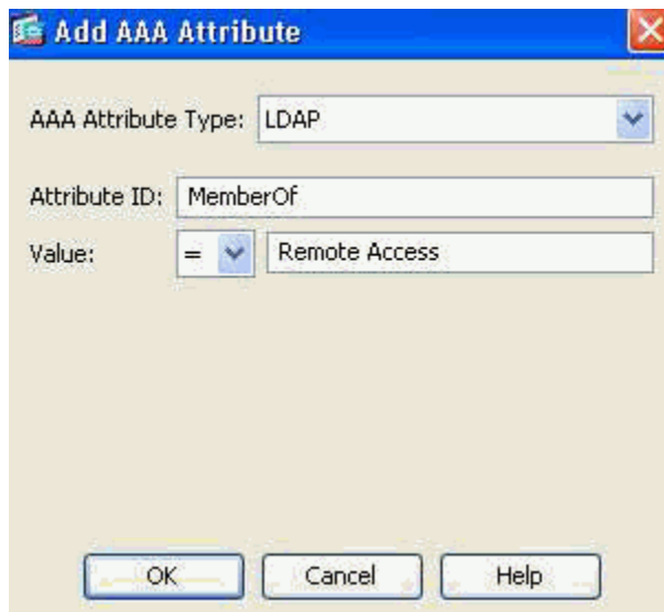
Figure 42. DAP AAA Attribute—AAA Group Membership will be used as a DAP criterion to allow remote access capabilities.
