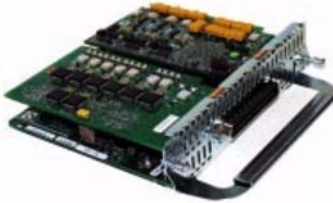
Figure 1. NM-HDA Network Module with 12 FXS Ports and 4 FXO Ports
