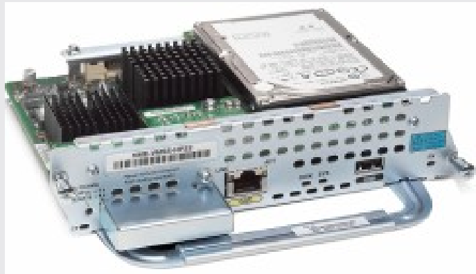
NME-VMSS: Video Management and Storage System
