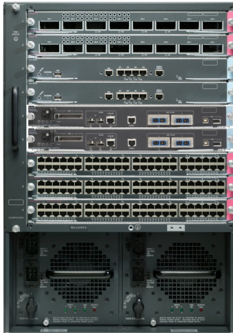
VSS Chassis with Dual Supervisors Running Quad-Sup Forwarding
