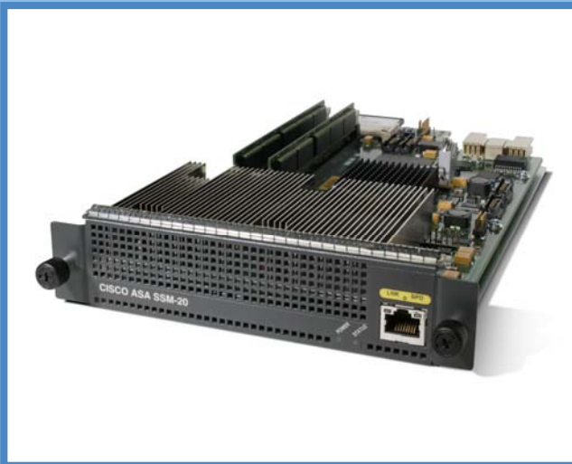
Cisco ASA 5500 Series Content Security and Control Module (CSC SSM)
