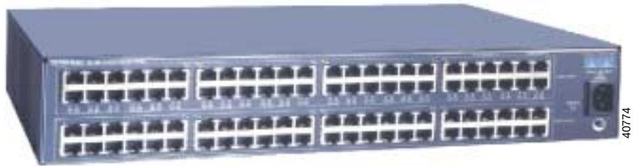
Abbildung 2-6 Cisco Power Patch Panel
