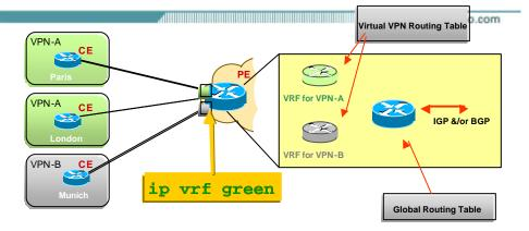
• Multiple routing & forwarding instances (VRFs) provide the separation
