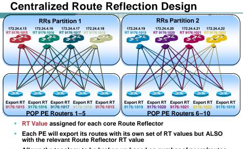
• Allows the topology to be broken up based on number of peers/routes rather than any specific RT values which would be difficult to manage Mpls\_vpns\_12\_01 ©2001, Clsco Systems, Inc. All rights reserved.
