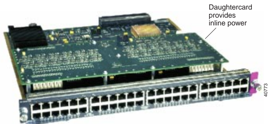
Figure 2-5 Catalyst 6000 Power-Enabled Line Card
