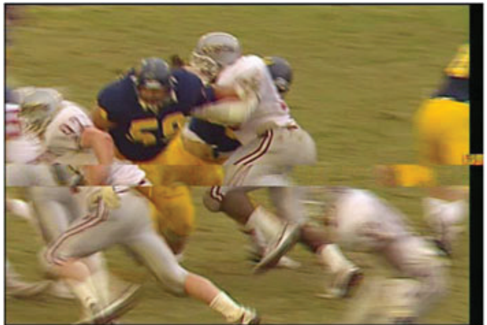
Figure 9. MPEG-2 Video GOP-Based Compression with a Slice Error Due to Packet Loss*
