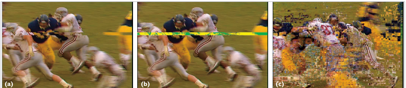
Figure 1. Video artifacts. With a slice error, we can see the image (a) as a viewer would see it and (b) with the parts in error highlighted. With a blocking or pixelization error (c), the effect occurs when a loss occurs in either an I- or P-frame. (Source material copyright the Society of Motion Picture Television Engineers, used with permission.)
