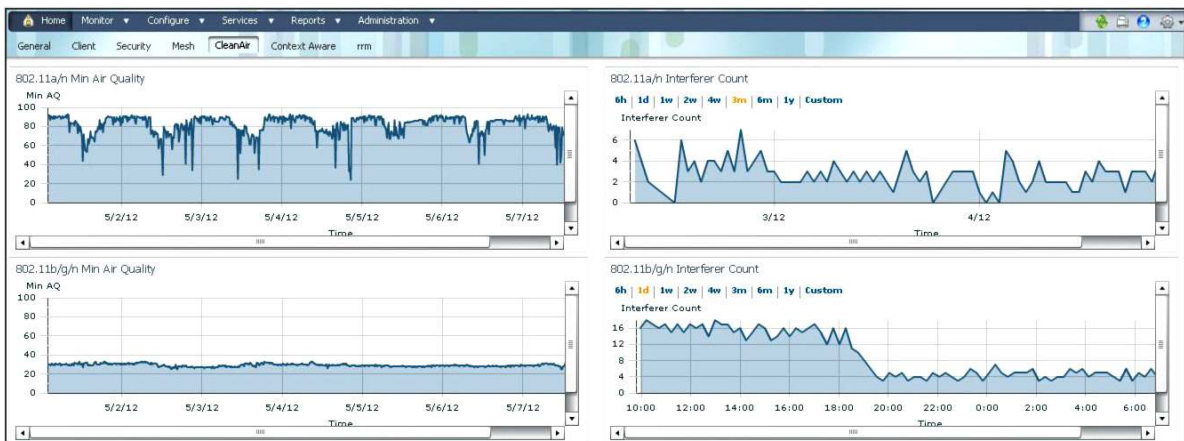
Figure 2. Monitoring Interference Devices, Air Quality Trends, and Alerts in the Cisco Prime Network Control System
