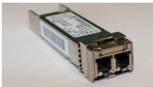
Figure 1. The SFP+ form factor allows higher densities
