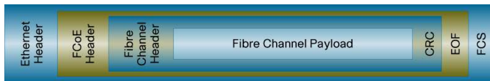
Figure 2. Encapsulation of Fibre Channel Frame in an Ethernet Packet
