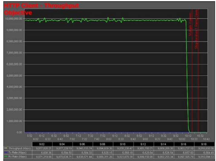
Figure Four: The Cisco ASR 1006 acquired an outstanding 9.98 Gbps throughput traffic, with no packet loss, with firewall enabled.
