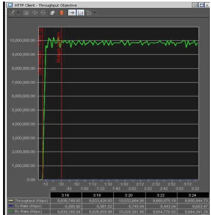
Figure Two: The Cisco ASR 1610 achieves up to 10 Gbps of routed throughput with no packet loss during the performance test.
