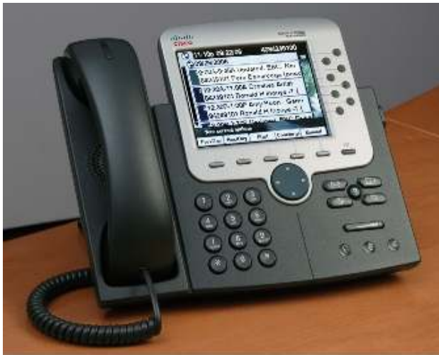
Figure 2. Meetings Posted on Cisco Unified IP Phone 7970G Display for One-Button-to-Push Call Launch
