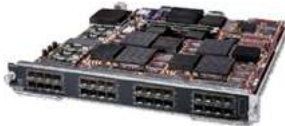
Figure 1. Cisco MDS 9000 Advanced Services Module
