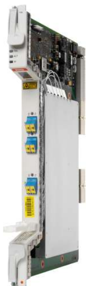
Figure 2. Channel Protection (Fiber Switched Protection)
