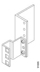
• Attach two adapters for racks with depths of 24 1/4 to 25 3/8 inches. Make sure the longer bracket is at the rear. Attach the two brackets to each other by using two cage nuts and two screws. See the following example.
