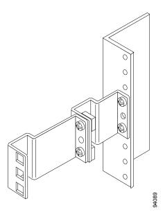
**Step 4** Attach a slide assembly to the adapters on each side of the rack:
