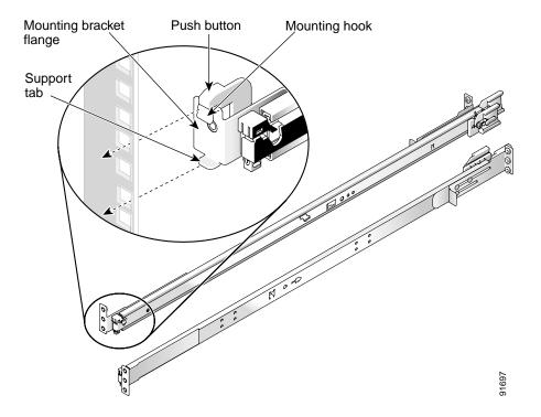
Step 5 Install the WLSE in the slide assembly.
