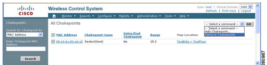
Figure 7-12 Removing a Chokepoint
