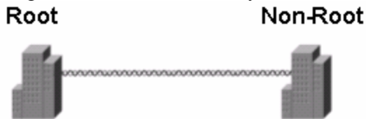
Figure 23. Point-to-Point Bridge Link
