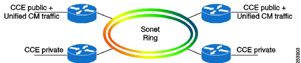
Figure 26 Network Architecture Based on a SONET Ring Under Normal Operations
