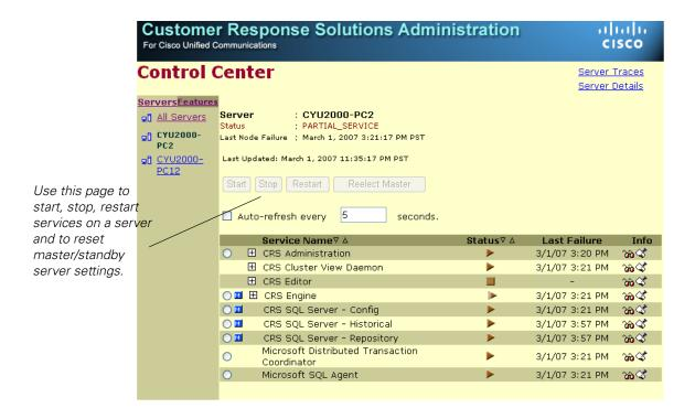
The Control Center configuration page lists the status of services running on a particular server; the figure above shows the status of services on a server named **PC22000**.
