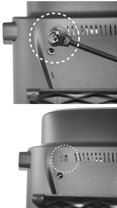
Figure 3-3 Connecting a Cable Lock to the Cisco Unified IP Phone 79761G/7961G-GE and 7941G/7941G-GE
