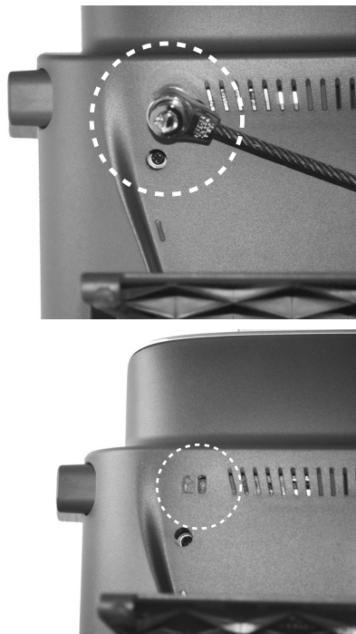
Figure 3-2 Connecting a Cable Lock to the Cisco Unified IP Phone 7961G/7961G-GE and 7941G/7941G-GE
