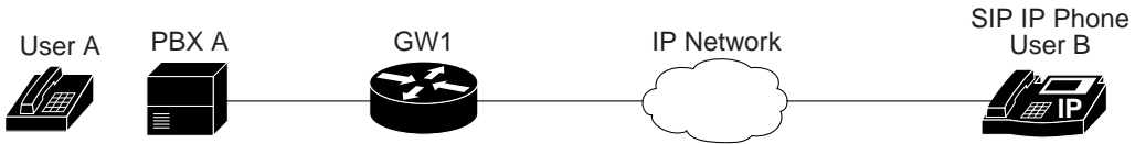
Figure B-2 Gateway-to-Cisco SIP IP Phone Call—Successful Call Setup and Call Hold
