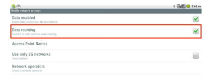
If wanting to preserve battery life / reduce battery usage, **Use only 2G networks** can optionally be enabled, where Cisco Cius SP will connect to an EDGE (2G) mobile network.
