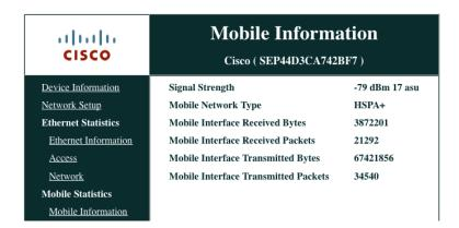
When connected to EDGE (2G), the signal strength, mobile network type and packet counts will be displayed in the **Mobile Information** section of the Cisco Cius SP webpage.
