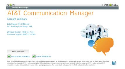
**Data enabled** in the mobile network settings must be selected in order to be able to connect to a mobile network.
