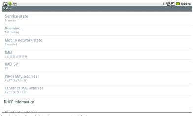
When not connected to a mobile network, the **Service state** will be displayed as **Out of service** in the **About Cius > Status** menu.
