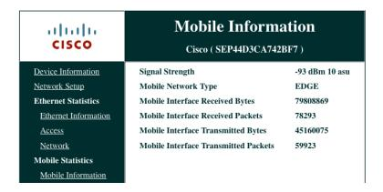
When not connected to a mobile network, there will not be any information for signal strength, mobile network type and packet counts displayed in the **Mobile Information** section of the Cisco Cius SP webpage.
