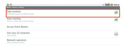
**Data roaming** in the mobile network settings must be selected in order to be able to connect to other service provider's mobile networks.
