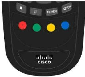
Each color can be assigned to a channel as a shortcut for a quick channel change. For example, if you assign the red button to channel 1, pressing the red button while watching a different channel at anytime will automatically tune the D9865 to TV channel 1.
