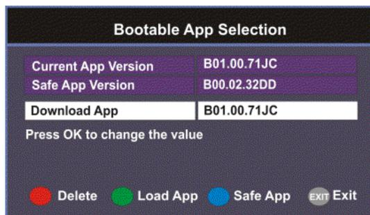
The **Current App Version** displays the currently running loaded application version number. The **Safe App Version** displays the factory loaded application version number.
