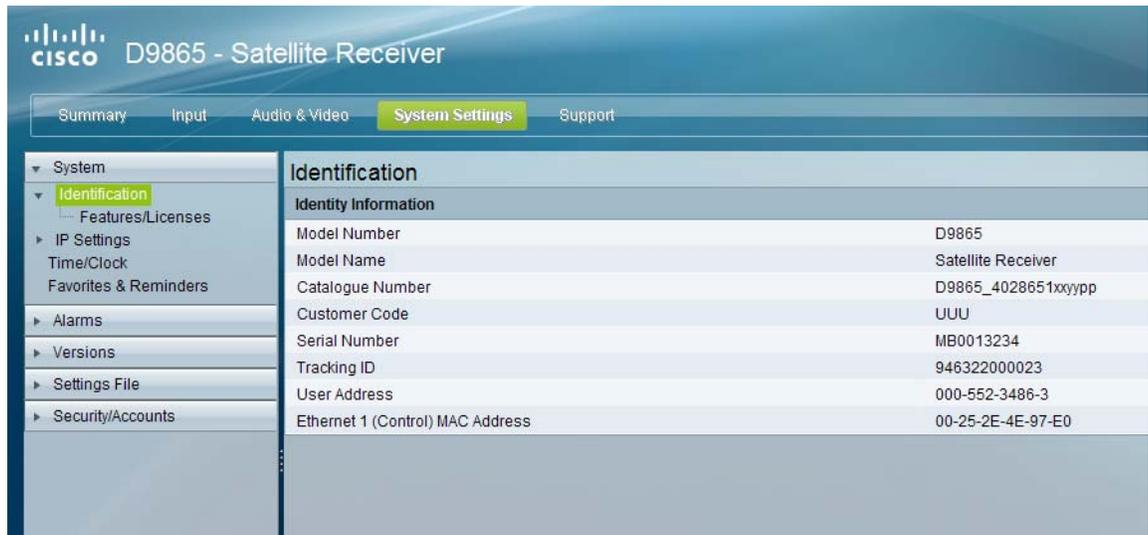
The Identification page displays the parameters associated with the D9865 system, such as model number, customer code, and user address. The following table displays the system information:
