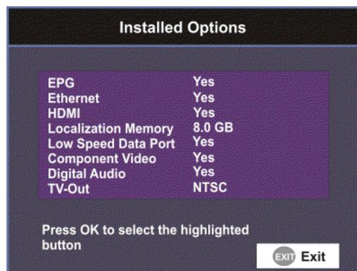
The Installed Options screen displays the hardware options installed in the current D9865 satellite receiver.
