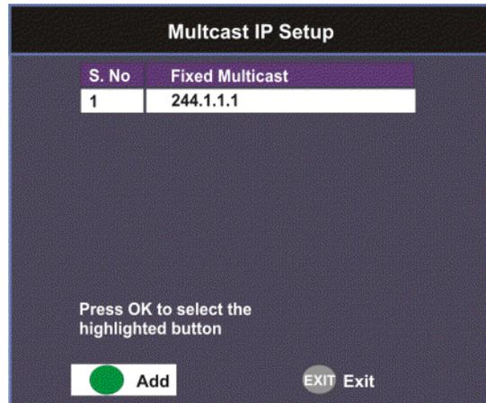
The Multicast IP Setup screen lists all the fixed multicast destination IP addresses.
