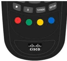
Enter a channel to each color as a shortcut for a quick channel change. For example, if you assign the red button to channel 1, pressing the red button while watching a different channel at anytime will automatically tune the TV channel to 1.
