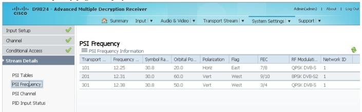
You cannot make any changes in the PSI Frequency table and can only view the available frequency plans stored in the receiver. The following is a list of the various columns:
