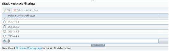
**2** Type the IP Address that sets the destination for multicast MPE data, in the range from 224.0.0.0 to 239.0.0.0.
