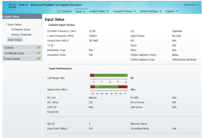
The **Current Input Status** area displays the same information shown in the Input Setup page. For more information on the parameters displayed, see *Setting up the RF Input* (on page 143).
