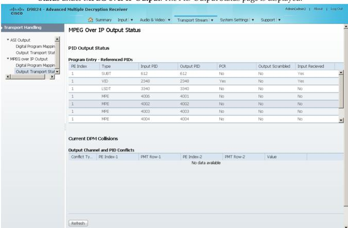
The **Program Entry - Referenced PIDs** table displays the specified PE ES PIDs information on the output.
