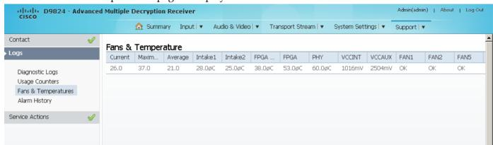
The **Current** column displays the current operating temperature. The **Maximum** column displays the maximum operating temperature that has been reached. The **Average** column displays the average operating temperature. The values are displayed in Degrees Celsius.
