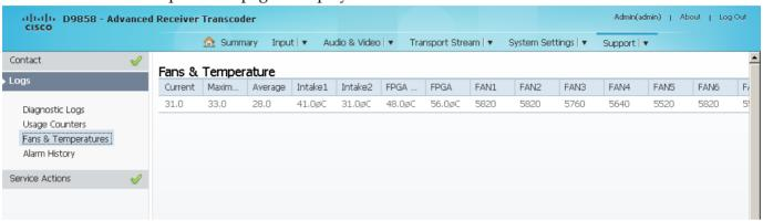
The Current column displays the current operating temperature. The Maximum column displays the maximum operating temperature that has been reached. The Average column displays the average operating temperature. The values are displayed in Degrees Celsius.
