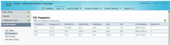
You cannot make any changes in the PSI Frequency table and can only view the available frequency plans stored in the receiver. The following is a list of the various columns:
