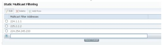
**2** Type the IP Address that sets the destination for multicast MPE data, in the range from 224.0.0.0 to 239.0.0.0.
