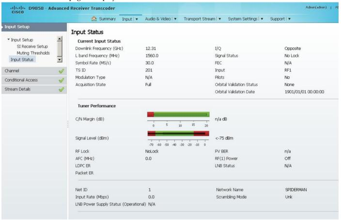
The **Current Input Status** area displays the same information shown in the Input Setup page. For more information on the parameters displayed, see *Setting up the RF Input* (on page 135).
