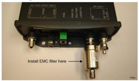
**Note:** Be sure to attach the EMC filter directly to the ONT RF port, ahead of any other cable to be attached to this port.
