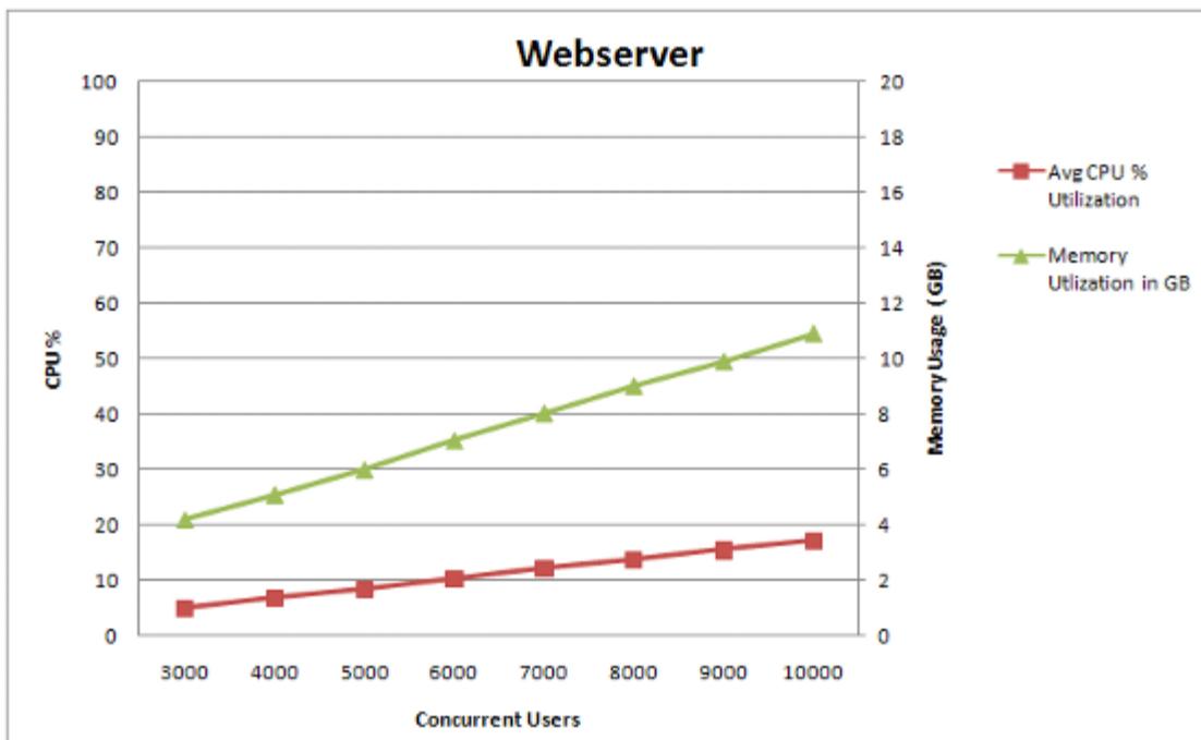
Figure 48 CPU and Memory Usage for Web Server
