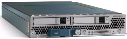
Figure 6 Cisco UCS B200 M2 Blade Server
