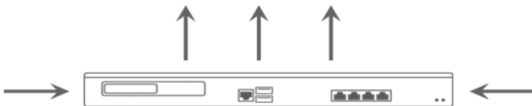
Figure 1: Cisco VCS ventilation
