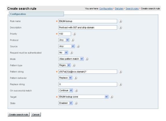
In this example, the search rule filters requests to the ENUM zone so that it is only queried for certain digit strings. A transform is also applied to remove any domain that may have been added by a SIP device or by a transform in the VCS to make E164 numbers into URIs.
