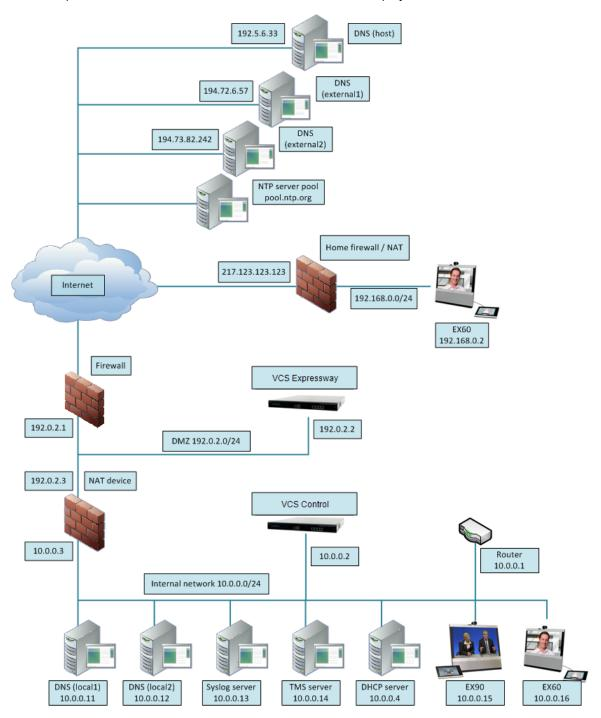
This example network includes internal and DMZ segments – in which VCS Control and VCS Expressway platforms are respectively deployed.
