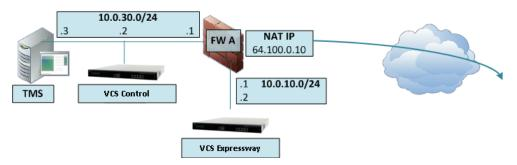
In this deployment, a 3-port firewall is used to create
