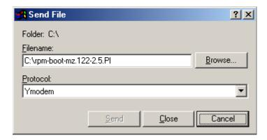
In the Filename box, browse and choose the image file to be downloaded. Also since we used the "y" option while invoking the xmodem, set the transfer protocol to ymodem or use Xmodem protocol by not specifying the –y option on the command line.
