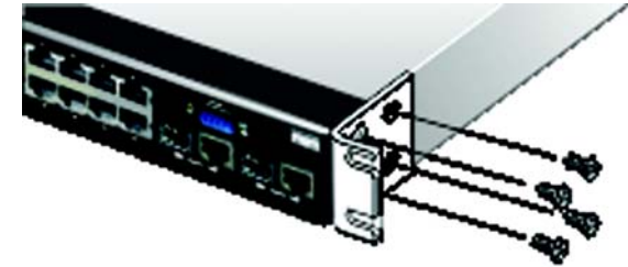
Figure 3-3: Attaching Brackets to the Switch
