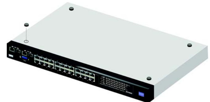
Figure 3-2: Attaching the Switch's Rubber Feet
