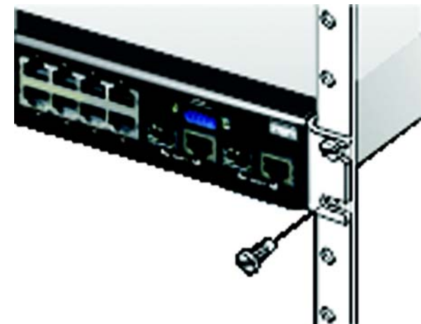
Figure 3-4: Mounting the Switch
