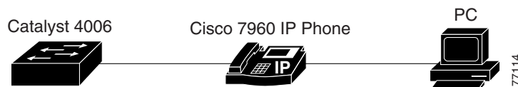
Figure 23-1 Cisco 7960 IP phone Connected to a Catalyst 4006 Switch with Supervisor Engine III
