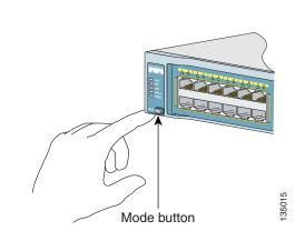
**Step 6** Verify that the switch is in Express Setup mode by confirming that all LEDs above the Mode button are green. (The redundant power system (RPS) and Power over Ethernet (PoE) LEDs remain off on some models.)
