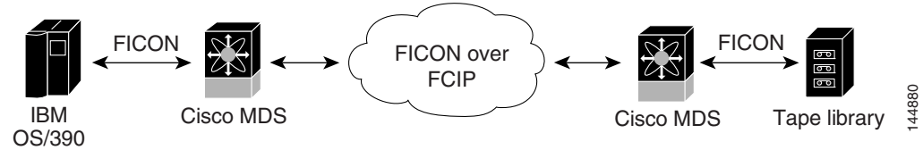
Figure 10-5 Host Directly Accessing IBM/STK (StorageTek) Library
