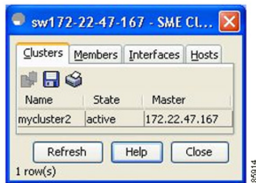
Figure 3-47 Viewing Cisco SME Cluster Information in Device View
