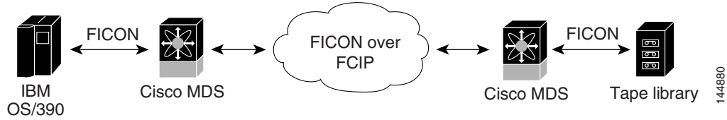
Figure 28-20 Host Directly Accessing IBM/STK (StorageTek) Library
