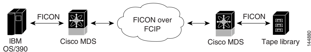
Figure 29-5 Host Directly Accessing IBM/STK (StorageTek) Library
