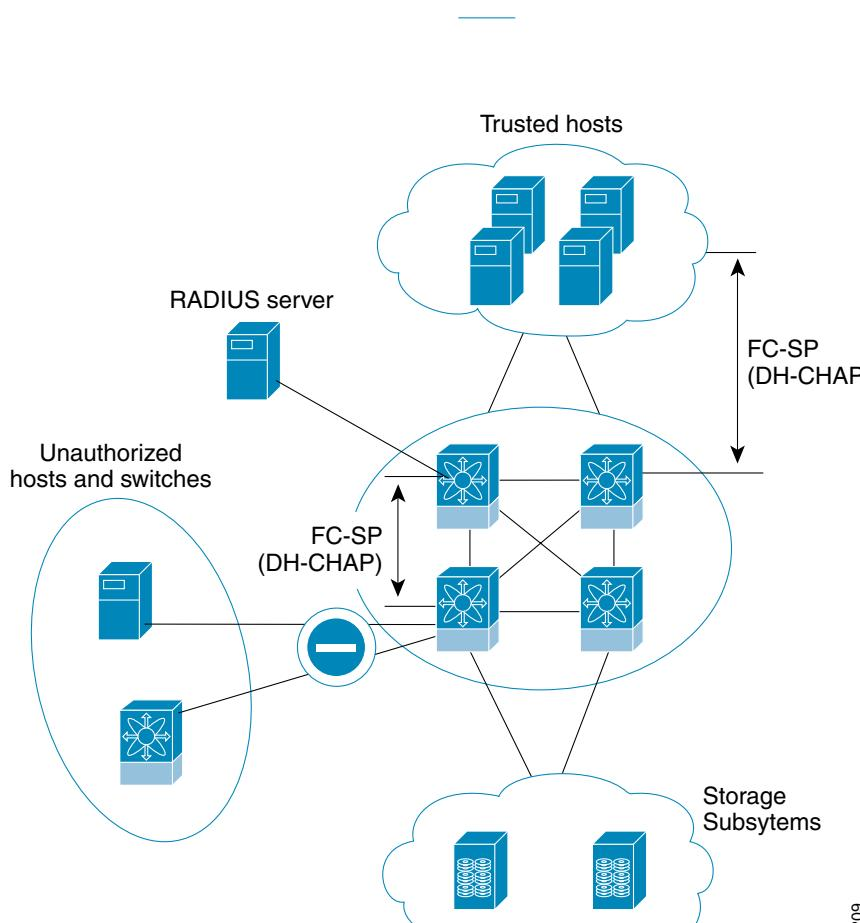
Fibre Channel (FC) host bus adapters (HBAs) with appropriate firmware and drivers are required for host-switch authentication.
