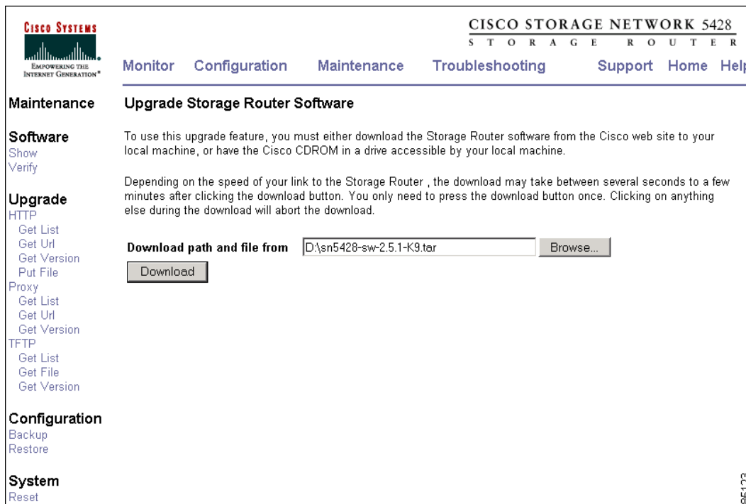
Figure 5 Upgrading via HTTP Put File
