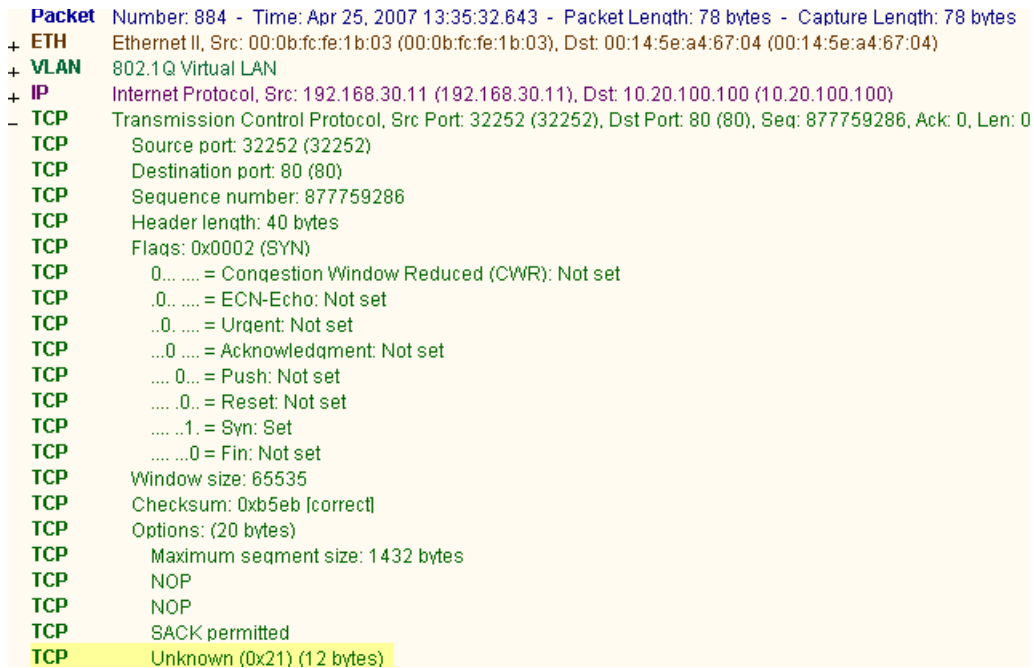
Figure 14 WAE TCP Option Trace
