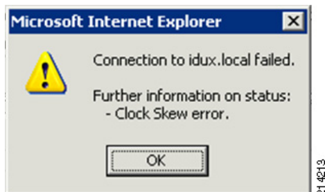
Figure 22 Connection Failed Message
