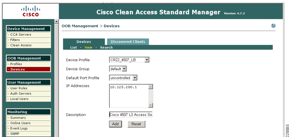
Figure 53 Adding Edge Switch in the NAC Manager to Control via SNMP
